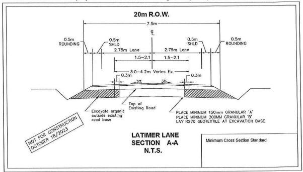
In addition to the required widening for the travelled portion, it was assumed that the shaded area shown above would have to be excavated and removed off site. The principle for this assumption is that the shoulders contain organic materials. Once that material has been removed, it will require new equivalent "B" and "A" materials to be placed on the road followed by re-ditching.
